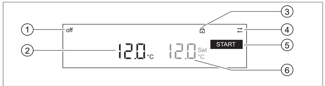
Fig. 4: Temperature display on the control panel
